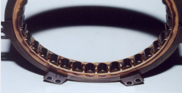
LM2500 bearing inspection shows excellent condition after 24000 hrs of operation in the oil & gas industry
