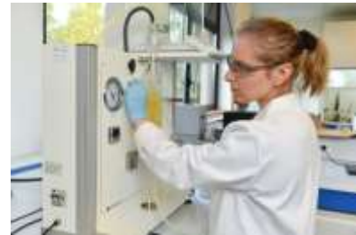
A technician doing a deaeration.
